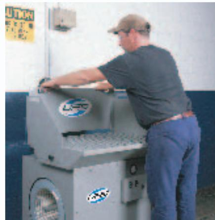
Panels can be easily removed for large parts.
