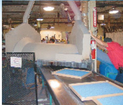
**UAS custom designed a hood to capture fiberglass dust directly at the source.**
